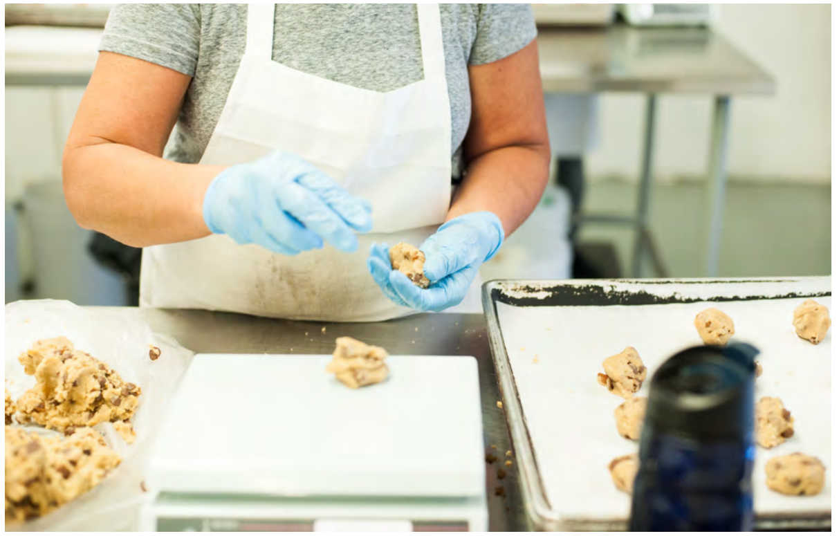
Each and every cookie produced at the Cookie It Up facility is formed and shaped by hand by one of several line operators from the freshly-mixed slabs of dough (above left) blended to right consistency on a nearby Hobart mixer.
